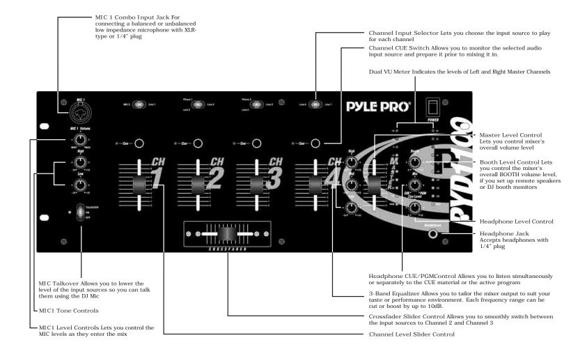
i - Pyle Pro Mixer Owner's Manual Pyle Pro Mixer Owner's Manual - 1 Presetting the Controls Before Use
